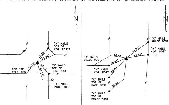
DISTANCES SLOPE CHAINED NW CORNER SECTION 18-82-41
