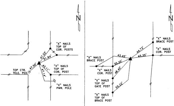
DISTANCES SLOPE CHAINED NW CORNER SECTION 18-82-41
