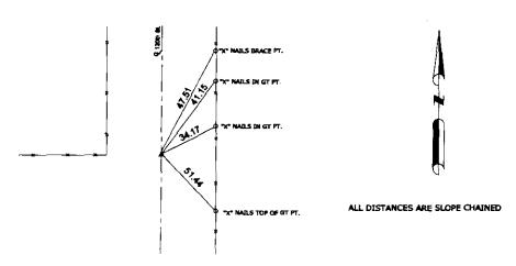
CORNER SET IN LINE WITH WEST FENCE AND 33' FROM ROAD FENCE TO EAST. CORNER IS ON & OF GRAVEL ROAD.
