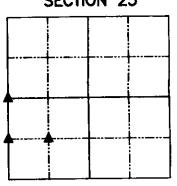
NW CORNER SW1/4 SW1/4 SEC. 25, T82N, R41W (Sat 5/8" dia. by 24" rebar w/arange cap PLS \$17048, 0.4' deep)
