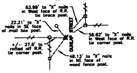
NE CORNER SW1/4 SW1/4 SEC. 25, T82N, R41W (Set 5/6" dia. by 24" rebar w/orange cop PLS \$17048, flush with surface)
