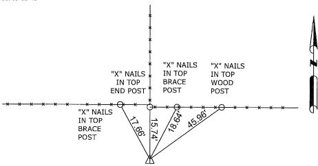
ALL TIE DISTANCES ARE MEASURED HORIZONTALLY USING GPS
