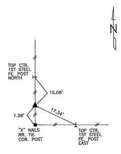
DISTANCES PLUMB CHAINED SW CORNER OF SE1/4 SE1/4 SECTION 33-82-41
