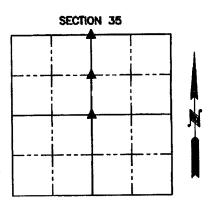
N1/4 CORNER SEC. 35, T82N, R41W (Set 5/8" dia. rebar w/orange cap PLS #17048, 0.5' deep on the Northerly slope of drainage ditch) 56.68° perp. to € of Hwy. 30.
