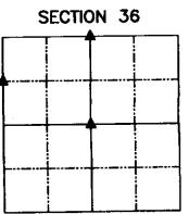
179'01'12" NW CORNER SEC. 36, T82N, R41W 1340.30'\_\_ 1328.58 ▲ N1/4 CORNER SEC. 36, TB2N, R41W (Fnd. concrete mon. 90'05'03" 88'25'24 w/brase disc in fence line 0.20' above surface) 8.55' West to "X" noils in South face of newer corner 1.90' East to West face of rotted off brace post. NE CORNER HW1/4 HW1/4 SEC. 36, TB2N, R41W 18 2528 SW CORNER NW1/4 NW1/4 SEC. 36, T82N, R41W (Set 5/8" dis. by 24" rebor w/orange cap PLS #17048, flush of with surface)
