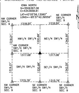
ALL DISTANCES PLUMB CHAINED NE CORNER SW1/4 SW1/4 OF SECTION 9-84-41
