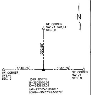
ALL DISTANCES PLUMB CHAINED SE CORNER SW1/4 SW1/4 OF SECTION 9-84-41
