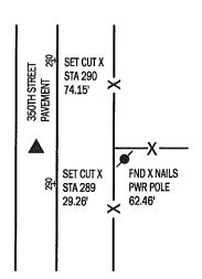
USED RECORDED TIES TO FIND LEAD PLUG AND VERIFY POSITION. ADDED CUT X'S TO THE STATION MARKERS FOR A MORE EXACT LOCATION, AND RETIED CORNER BECAUSE TIES TO THE WEST ARE NOW GONE.
