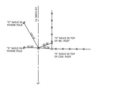
ALL TIE DISTANCES ARE HORIZONTAL DISTANCES MEASURED USING GPS
