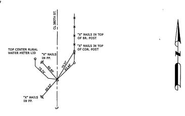
ALL TIE DISTANCES ARE HORIZONTAL DISTANCES MEASURED USING GPS
