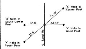
None of the ties obtained from the County Engineers Office checked out in the County Engineers Office checked out in the field. Checked for more Info at Engineers Office, nothing found on road plans, etc. Set SW corner from Existing Corner Posts, due to the fact that road plans stated the Section Line and Centerline were one. Aerials also showed the West 1/4 Cor as splitting the ROW. Did so and Set pin in line with Fence Line to the West.
