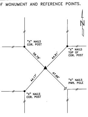
DISTANCES SLOPE CHAINED SE CORNER SECTION 10-82-38
