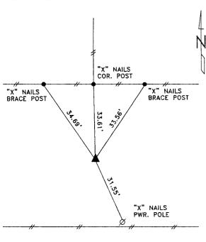
DISTANCES SLOPE CHAINED S1/4 CORNER SECTION 31-82-38
