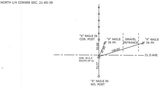
ALL TIE DISTANCES ARE MEASURED HORIZONTALLY USING GPS
