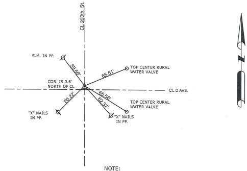
S.M. = SURVEY MARKER PLASTIC REFERENCE DISC ALL TIE DISTANCES ARE MEASURED HORIZONTALLY USING GPS
