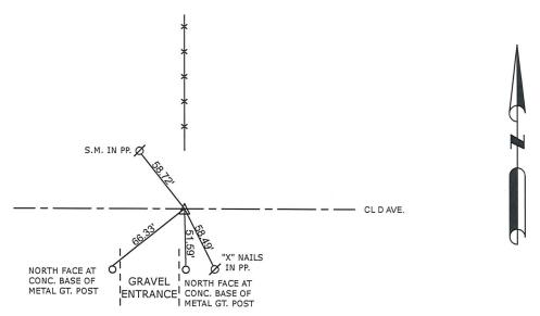
NOTE: S.M. = SURVEY MARKER PLASTIC REFERENCE DISC ALL TIE DISTANCES ARE MEASURED HORIZONTALLY USING GPS
