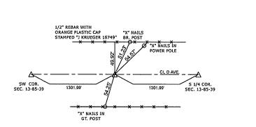
ALL TIE DISTANCES ARE MEASURED HORIZONTALLY USING GPS
