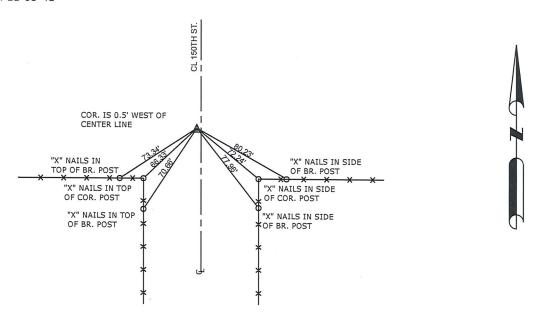
ALL TIE DISTANCES ARE HORIZONTAL DISTANCES MEASURED USING GPS
