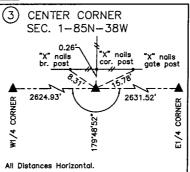
SET 5/8" DIA. x 24" REBAR W/ORANGE CAP PLS #17048 (FLUSH).
