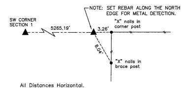
FOUND CONCRETE MONUMENT WITH THE TOP BROKEN OFF AND MISSING (1.0' DEEP).
