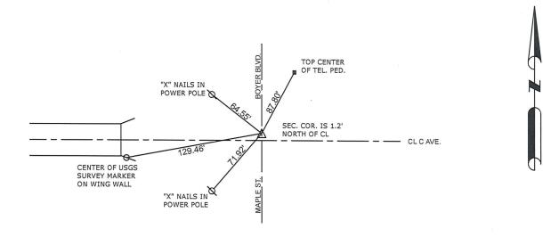
ALL TIE DISTANCES ARE MEASURED HORIZONTALLY USING GPS
