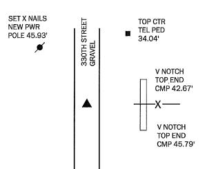
USED RECORDED TIES TO FIND 1" BOLT 0.40' DEEP. CHECKED TIES AND ADDED X NAILS TO A NEW POWER POLE. THE OLD POWER POLE HAS BEEN REPLACED SO TIES HAVE CHANGED SINCE LAST CERTIFICATE.
