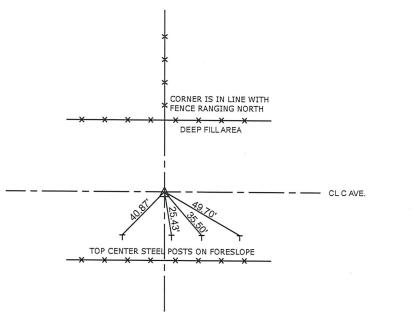
ALL TIE DISTANCES ARE MEASURED HORIZONTALLY USING GPS
