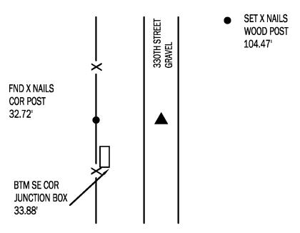
USED RECORDED TIES TO FIND 1/2" REBAR 4" DEEP. VERIFIED POSITION OF MONUMENT WITH EXISTING TIES. THE GATE POST ON THE EAST SIDE IS NOW GONE, SO AN ADDITIONAL TIE WAS SET TO A WOOD POST.
