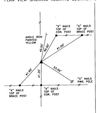
DISTANCES SLOPE CHAINED S1/4 CORNER SECTION 4-85-38
