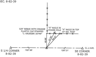
ALL TIE DISTANCES ARE MEASURED HORIZONTALLY USING GPS
