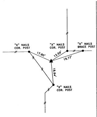
DISTANCES SLOPE CHAINED CENTER OF SECTION 9-82-39
