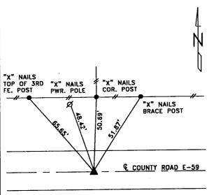
DISTANCES SLOPE CHAINED S1/4 CORNER SECTION 9-82-39
