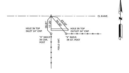
ALL TIE DISTANCES ARE MEASURED HORIZONTALLY USING GPS
